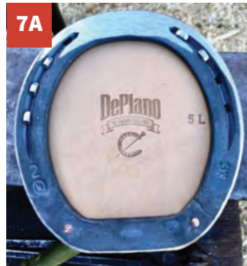
Fig. 7A and 7B. Kerckhaert SX-8 straight bar shoe with impression material. Note the space created between the hoof surface and the shoe.
