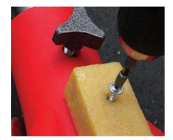
3. LAY THE HOOFJACK ON ITS SIDE, BRACE IT AND APPLY THE SELF-PIERCING SCREWS IN YOUR HOLES. MAKE SURE YOU TIGHTEN UNTIL THE HEAD IS SUNKEN INTO THE STICK ABOUT 3/4", NOT JUST FLUSH WITH THE OUTSIDE.
