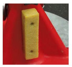
4. TWO SCREWS SHOULD BE ADEQUATE. MOUNTING BELOW THE TENSION KNOB IS THE BEST LOCATION.
