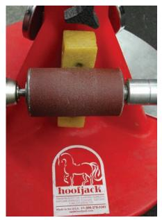
6. WHEN YOUR BUFFER SLEEVE GETS DIRT BUILDUP, SIMPLY RUN THE TOOL AND APPLY SLIGHT PRESSURE ON THE STICK. IT WILL CLEAN UP VERY QUICKLY.
