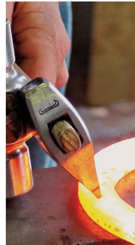
Forepunch to final depth, drift and pritchel.
