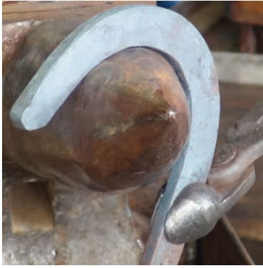
Turn branch over horn, striking the shoe just past the center of the horn to make the bend.
