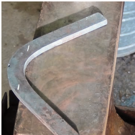
You can eyeball it or use a Bloom t-square tool to mark your toe nail.
