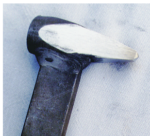
6. Put point on all forepunch ends. Right: Maintained and ready to go back to work.
