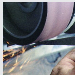
9. Pritchel with broken tip. Grind end flat. Grind to desired dimension. Use this approach to the wheel for aggressive stock removal.
