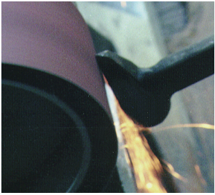
4. Grind back to desired nail dimension.
