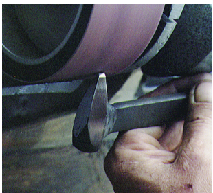
6. Put point on all forepunch ends. Right: Maintained and ready to go back to work.
