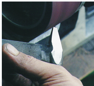
5. Check against nail or use a guide. This one is made from aluminum.
