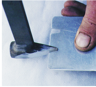
5. Check against nail or use a guide. This one is made from aluminum.
