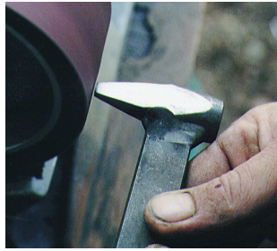
4. Grind back to desired nail dimension.
