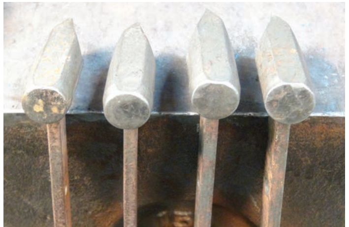
FOUR TOOLS ALL USED IN CROSSOVER STYLE. TWO TOOLS USED BY RIGHT HANDER, TWO BY LEFT HANDER. IF YOU LOOK CAREFULLY YOU CAN SEE ALL WERE STRUCK OFF CENTER.
