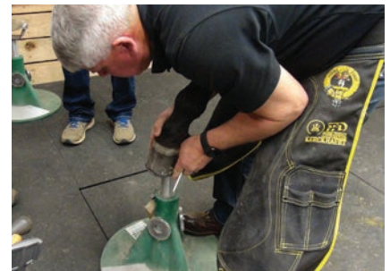
Checking the fit of the shoe and marking any needed grinds is another great use of the stand.
