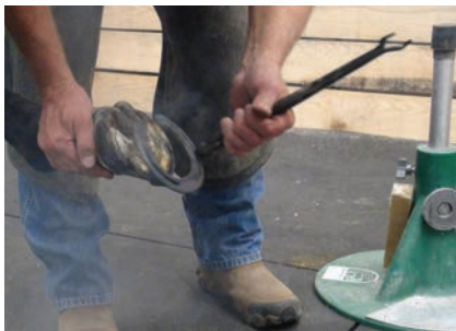
Hot fitting off the stand but notice the aluminum plate modification on the Hoofjack base used to set the hot shoe on while final paring the sole.
