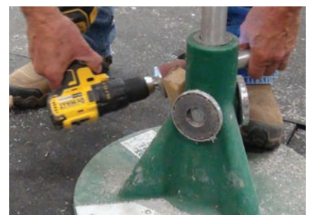
Attach a rubber cleaning stick to the Hoofjack to clean the sanding sleeve on a FootPro Hoof buffer to keep it in good working order.
