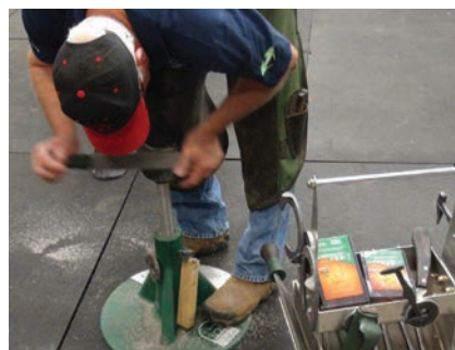
Whether you are using a rasp/file or a buffer, having the foot on a stand takes a lot of pressure off your back and legs.
