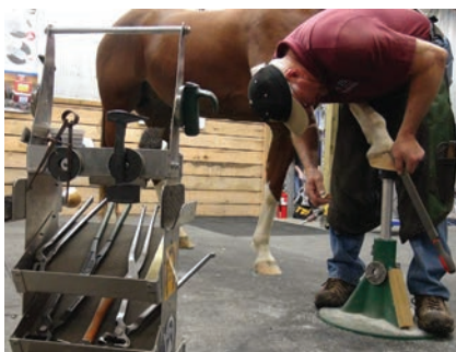
Putting the foot up on the stand allows you to take a good look at flares and the finish of the outer wall.
