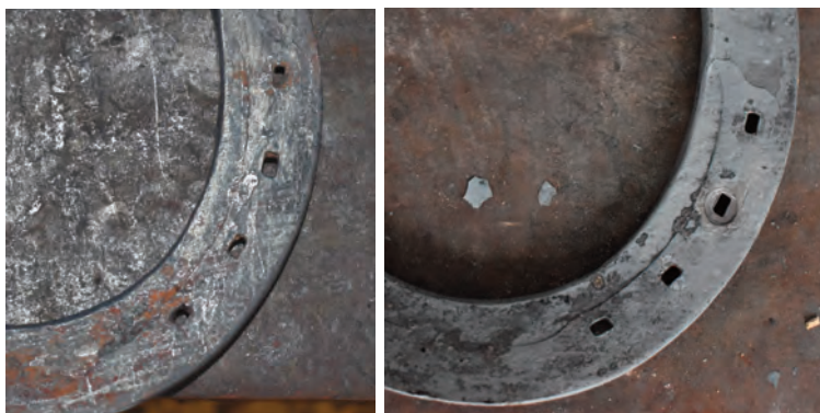
Left: Reset. Right: Repaired worn nail hole for proper nail fit on reset. Note that I lightly drive a stud punch into the foot side of the shoe at low heat.
