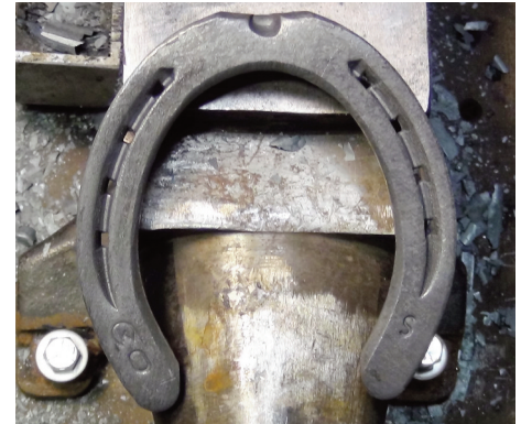
Finished clip from ground surface.
