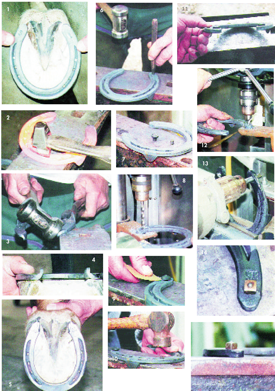
1. Factory rim style shoe, creased through toe. 2. Plain factory shoe being creased through toe. 3. Making in-line jar calk by turning inside of heel at edge of anvil. 4. In-line jar calk. 5. In-line jar calk positioned on foot. 6. Center punch your drive-in or screw-in calk positions. 7. Two common sizes of drive-in studs. 8. Drilling is all that's necessary for the drive-in calks. Most have tapered shanks. 9. When driving in studs with head, be sure not to bottom out, leave a slight gap between shoe and shoulder of stud. 10. Use a steel hammer with an annealed face to avoid injury from chipping. 11. Smaller studs driven flush used in toe with slightly taller studs in heels. 12. When drilling for screw-in calks be sure to countersink. This makes application much easier. 13. Use appropriate tap for the screw-in calks you will be using. 14. Screw-in calks should normally not be placed at end of heel. Slightly more forward than the studs in this photo would probably be preferable in most cases. 15. Two different size calks. Choice will usually be made based on surface conditions.
