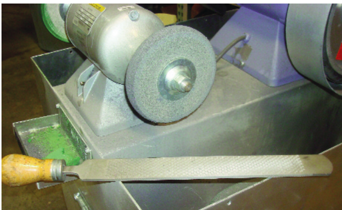
ABOVE: AN OLD RASP IS THE ONLY TOOL NEEDED.
