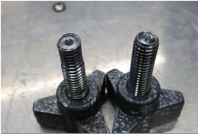
NEW TENSION KNOB (RIGHT) COMPARED TO HEAVILY WORN TENSION KNOB (LEFT). THIS IS AN EXTREME EXAMPLE THAT DOES NOT REFLECT NORMAL WEAR AND TEAR.
