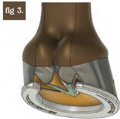
A foot shod with a conventional shoe is an extension of the hoof wall. There is an increased load on the hoof wall, and heels are loaded more, the frog and bars are elevated and loaded less.
