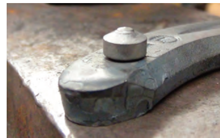
C11 applied – note the small gap between head and shoe surface.
