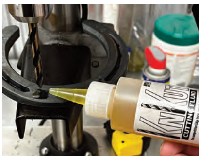
Cutting Fluid applied before drilling
